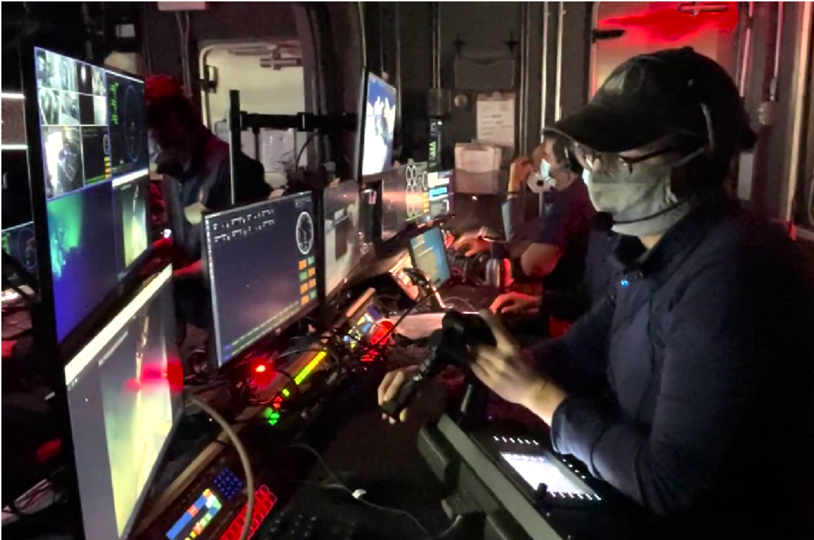
Figure 1-1: Photo of an ROV pilot operating an ROV manipulator arm from an onboard control room with the conventional topside controller. Conventionally, pilots complete dexterous sampling tasks using this controller with support from numerous telemetry and video feeds. (Image credit: Matthew Walter)
