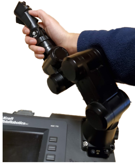
Figure 4-1: Photo of the conventional topside controller used to control the hydraulic manipulator arm during user testing
